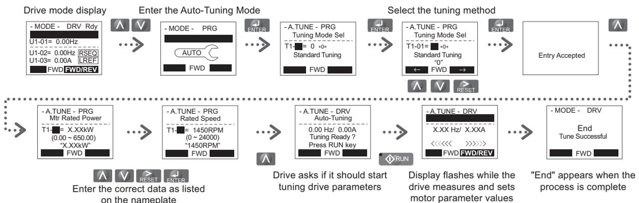
If Auto-Tuning cannot be performed for some reason (no-load operation impossible, etc.), then set the maximum frequency and voltage in the E1-□□ parameters and enter the motor data manually into the E2-□□ parameters. Refer to *Auto-Tuning Errors on page 41*.
