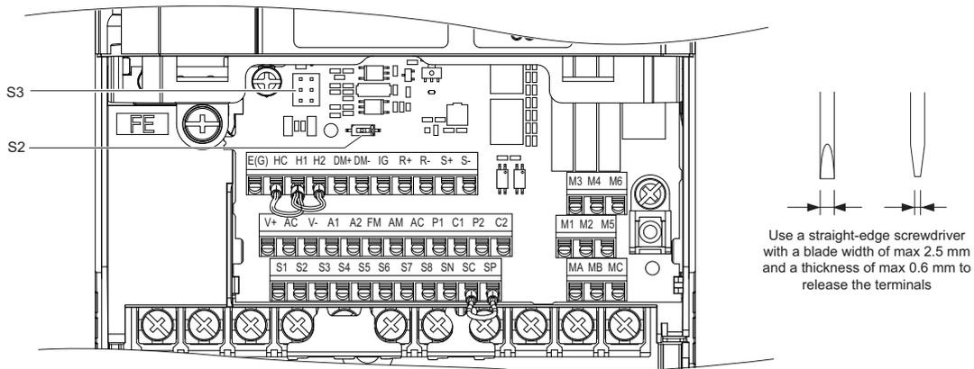
DIP switch S2 and jumper S3 are located on the terminal board. Set them as described below.
