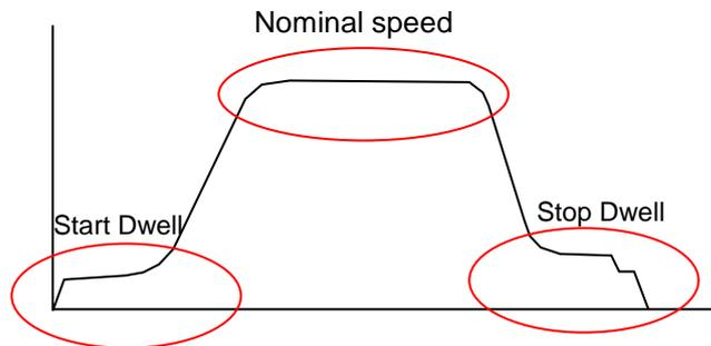
**1) START UP: As motor starts running at first the lift moves suddenly up then accelerates smoothly**
