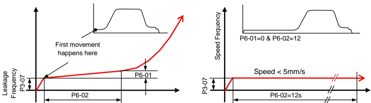
**d) Adjust P3-07 (leakage frequency) so that lift moves upwards (EMPTY) very slowly about 5mm/s (=0.005m/s) or less during the initial 12s.**
