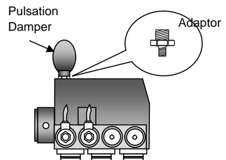
**How?** Close the ball valve → Turn emergency lowering to relieve the pressure → Remove the plug from the **Z1** port → Connect the pulsation damper to the valve by using 1/4" to 1/2" adaptor with copper washers.
